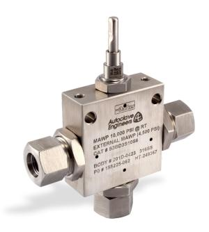
The Parker Autoclave Engineers ball valves can be utilized to switch or isolate flow. The standard material of construction of the valve is 316 cold worked 316/316L with PEEK seats, graphite filled PTFE stem seal, and o-ring material as required by the process fluid.
